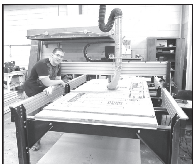
Photo by Mark Harper Kevin Harney of Mr. French’s shop class, oversees the progress of the Shop Bot as it cuts out each side of a sawhorse.
