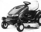
SST18 Lawn Tractor • 18-hp. V-Twin engine • Two-pedal automatic transmission 48-inch mower deck • Zero-turn radius with power steering
